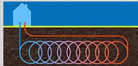
Ground sourced heat pump (source: PUSH doc)
